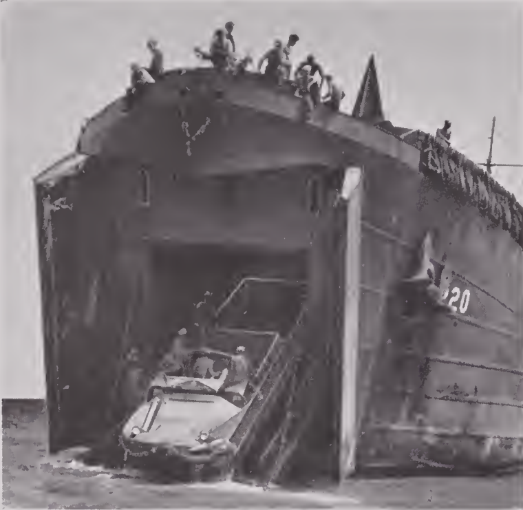
FIGURE 8. DUKW discharging from tank deck of LST into sea. This technique is incorrect. DUKW should be loaded on bow first so that it will back off, thus avoiding the possibility of damaging pintle hook, propeller guard, or propeller.
